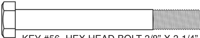
KEY #56 HEX HEAD BOLT 3/8" X 3 1/4" PARTIAL THREAD QTY. 2
