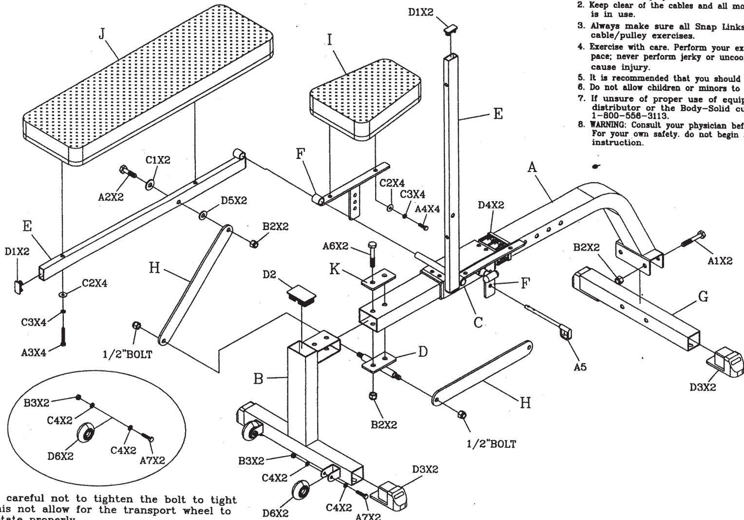
\*Be careful not to tighten the bolt to tight. This not allow for the transport wheel to rotate properly.
