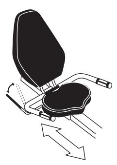
Grasp the Seat Adjustment Knob, located at the base of the seat post. Turn knob to lossen then pull out and raise or lower the seat post to the desired height . Release the knob and turn knob to tighten to allow the seat post to lock into position.
