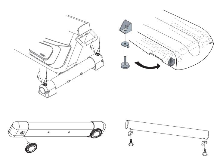
Note: adjust for leveling screws as neccessary prior to use.
