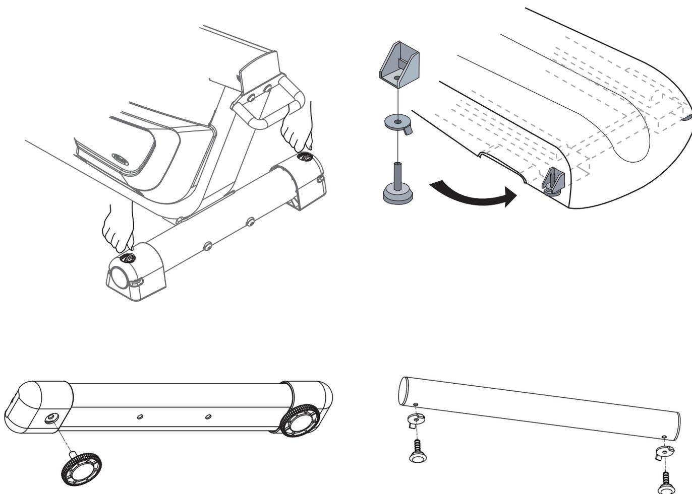
Note : adjust for leveling screws as necessary prior to use.
