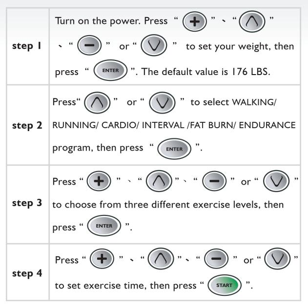
Center Display counts down 3 seconds, and then starts belt. During your workout, you can change speed and incline using Quick Keys, corresponding arrow or "+" "-" keys.
