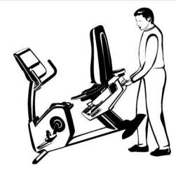
To move PR10, firmly grasp rear handlebar, carefully lift and roll on transport wheels.
