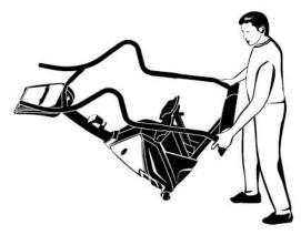
To move PST10, firmly grasp bottom areas of handlebars, carefully lift and roll on the transport wheels.
