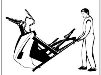
To move PESG/PE10, firmly grasp assembled rear foot, carefully lift and roll on transport wheels.
